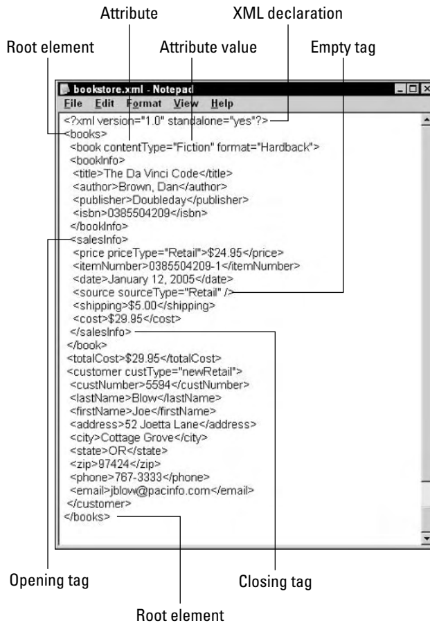
Figure 5-1: Dissecting the different parts of a well- formed XML document.
