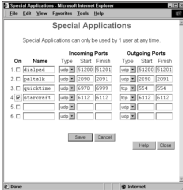
Figure 12-3: Setting up port forwarding.
