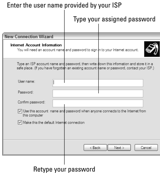
Figure 2-9: When creating a new dial-up connection, enter the user name and password provided by the ISP.
