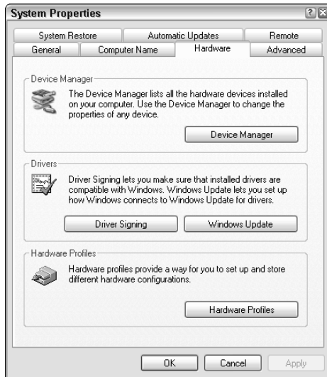
Figure 1-1: To find out if you have USB 1.1 or 2.0, look in the Device Manager.
