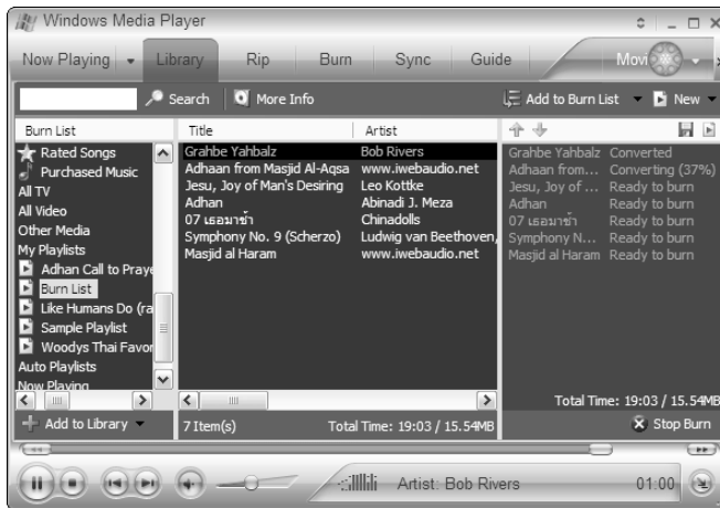
Figure 1-28: Before writing the tracks to a CD, WMP converts them to a format that plays on a CD player.
