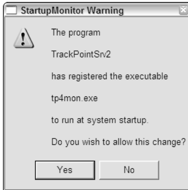
Figure 3-5: Startup Blocker lets you know if a program is trying to set itself up to run automatically every time you start Windows.
