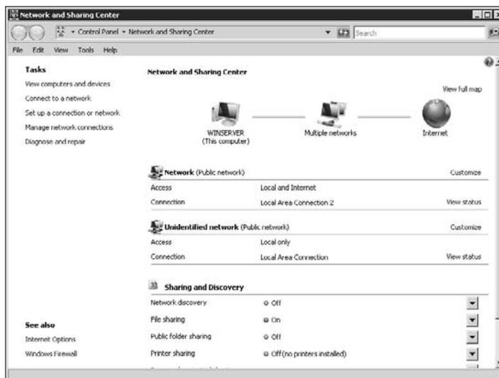
Each of the NICs in your system receives a connection entry in the Network and Sharing Center. The network information includes the network type (public or private), the network name, and the connection name. The connections also contain two links: Customize and View Status.
