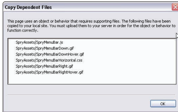
Figure 6-14: Be sure to upload the special SpryAssets folder to the server along with your Spry menu pages to ensure that your menu functions properly.
