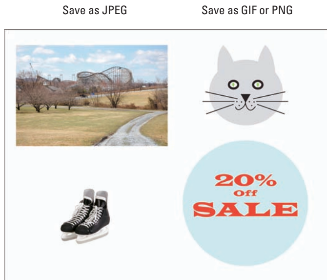
Figure 3-8: Optimize your Web graphics with photographs and gradients as JPEG and all others as GIF or PNG.
