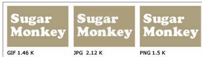
Figure 3-10: Save images with large, flat areas of color and text as a GIF or PNG for best results.
