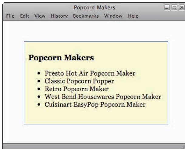
Figure 3-9: ID styles in the CSS are automatically applied to objects on the page with the same ID.
