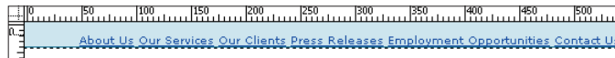
Figure 6-19: Styling the <li> tags gives your CSS navigation system a horizontal layout.
