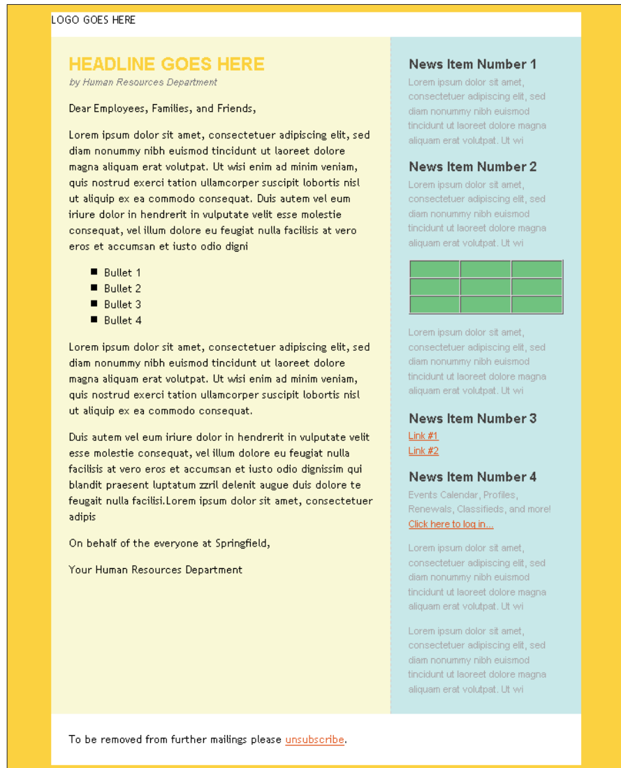
Figure 5-6: Stack and nest tables to achieve a layout that matches your design.
