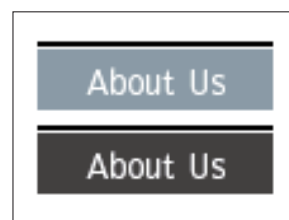
Figure 6-9: Rollover buttons need two graphics: one for the normal state (top) and another for the over state (bottom).
