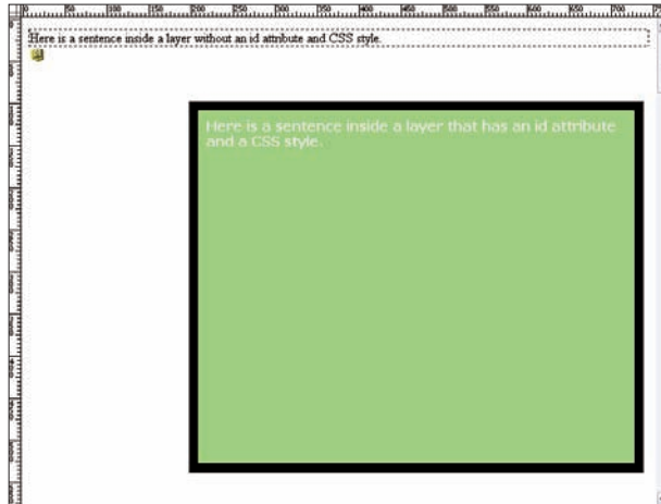
Figure 5-2: Add a CSS style to your layer to control the layer's look and position.
