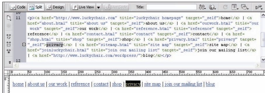
Figure 9-6: SSI files can be updated in an HTML editor just like regular HTML files.
