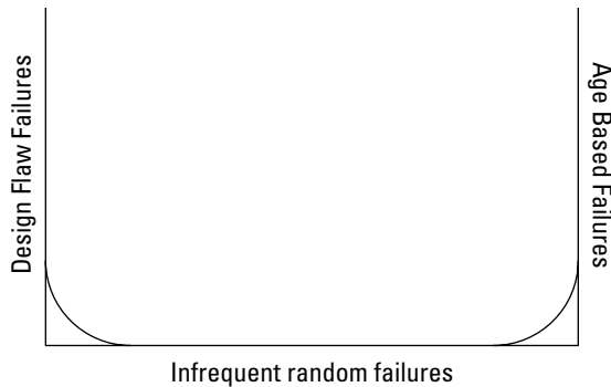
Figure 8-2: Disk failures follow the bathtub curve.
