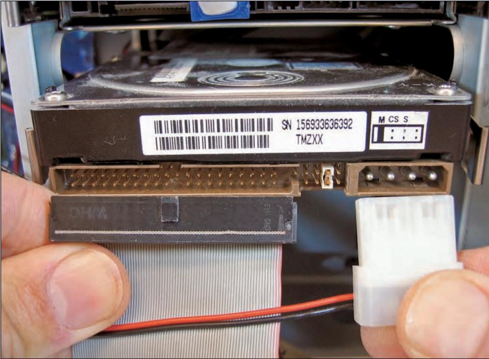
**Color Plate 24:** Plug two cables into an IDE drive, whether it's a hard drive or CD/DVD burner. The other end of the data cable (left) plugs into the motherboard. The power cable (right) extends from your power supply.
