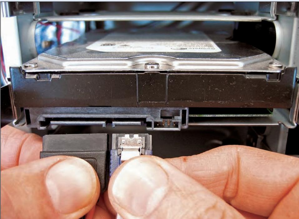
**Color Plate 25:** Plug two cables into the SATA hard drive. The data cable (right) plugs into the motherboard. The power cable (left) extends from your power supply.
