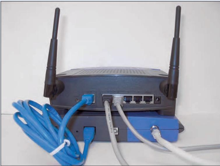
**Color Plate 28:** Connect the round cable to your cable modem. Connect an Ethernet cable between your cable modem and the port on your router that's labeled "WAN." Then plug your PC's Ethernet cables into your router's numbered ports.
