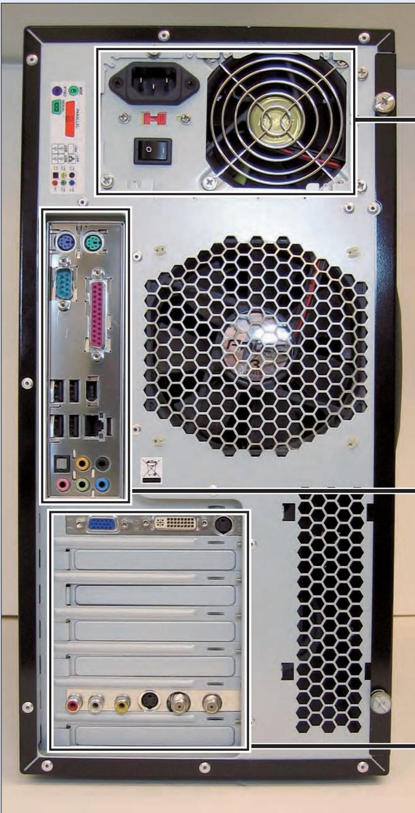
**Color Plate 4:** On the back of every PC, you see the power supply, the ports, and the slots.
