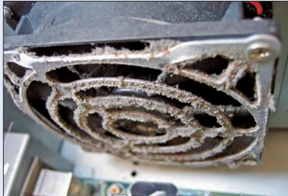
**Color Plate 33:** Don't let dust collect inside your PC. And when blowing off the dust with compressed air, do it outdoors, so the dust doesn't fill your lungs and get all over the room.
