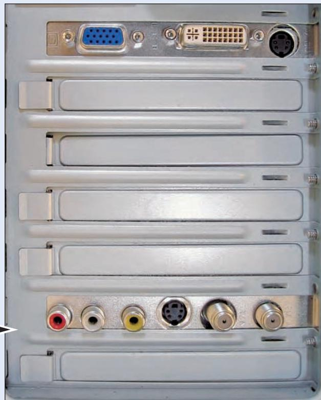
**Color Plate 7:** The back side of your PC's cards poke out the back of slots cut into the rear of the PC's case. (The bottom card is a TV tuner card; the top is a video card.)
