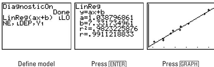
Figure 19-8: Steps for calculating and graphing a regression model.
