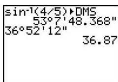
Figure 3-5: Converting between degrees and DMS.
