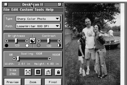
Figure 5-5: The marquee box lets you crop a preview image to make it smaller and reduce the file size.
