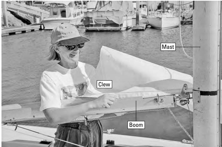
Figure 4-8: Sliding the mainsail foot rope into the track on the bottom.
