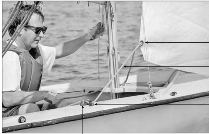
Figure 4-11: Jib sheet system on a 420-class dinghy.
