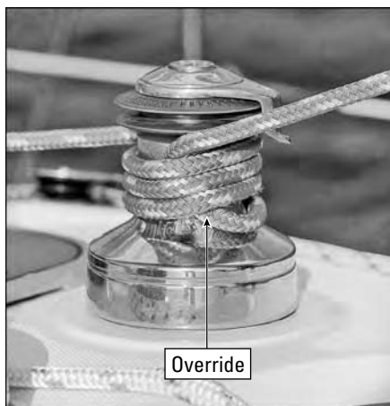
Figure 5-18: An override (left) and a properly wrapped winch (right).
