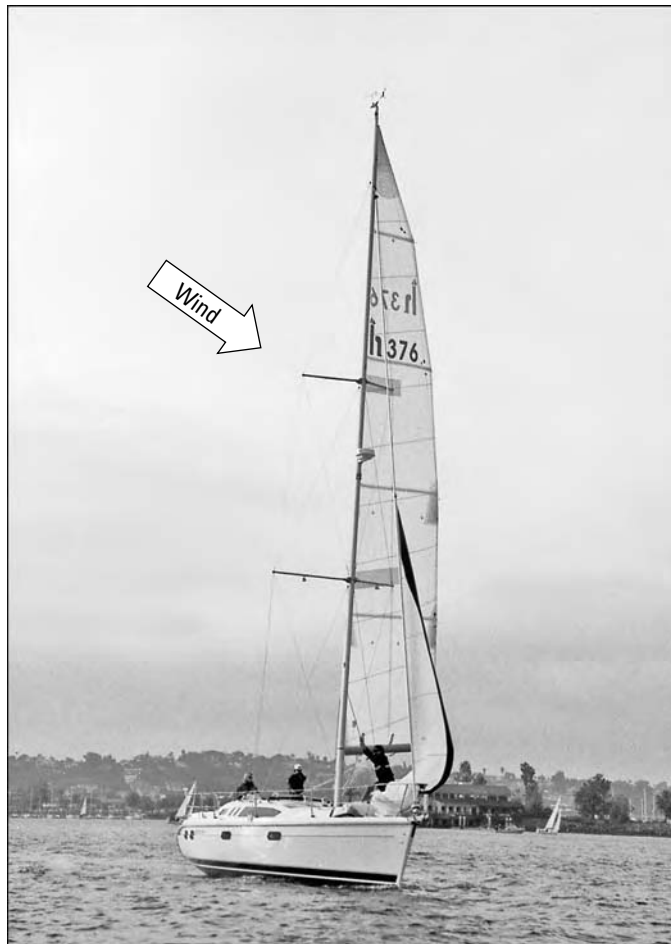
Figure 4-15: Hoisting the jib while under way and pointing downwind.
