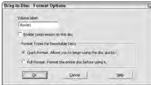
Figure 3-4: The Disc Format options dialog box appears whenever you manually format a blank disc.
