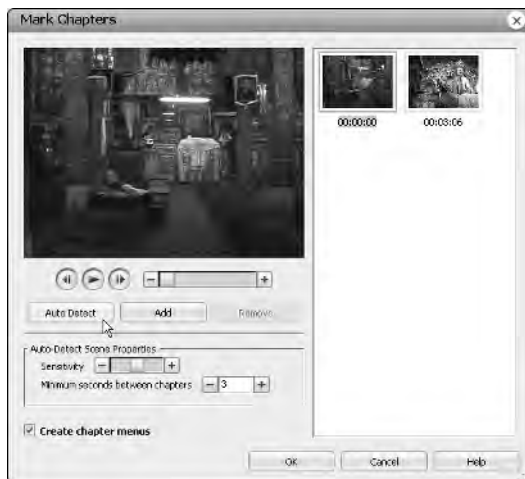
Figure 11-10: You use the controls in the Mark Chapters dialog box to add, change, or delete chapter markers in the current title.
