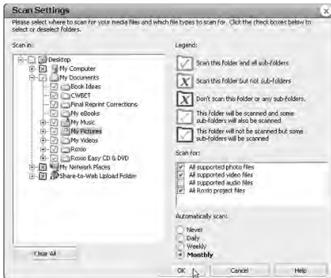
Figure 4-4: Adjust the options in the Scan Settings dialog box as needed to determine which folders are scanned how often for what types of files.
