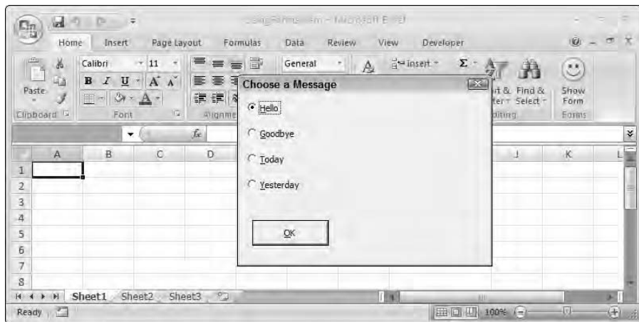
Figure 4-6: Forms let you provide extra options that don't appear on the Ribbon.
