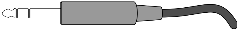
Figure 2-5: A \frac{1}{4} -inch male connection, the connection needed to connect headphones to a mixing board.
