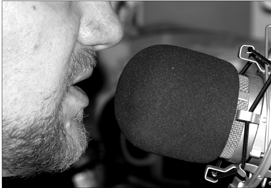
Figure 4-2: Set your microphone at a comfortable distance, close enough to overpower ambient noise, but avoid microphone contact.
