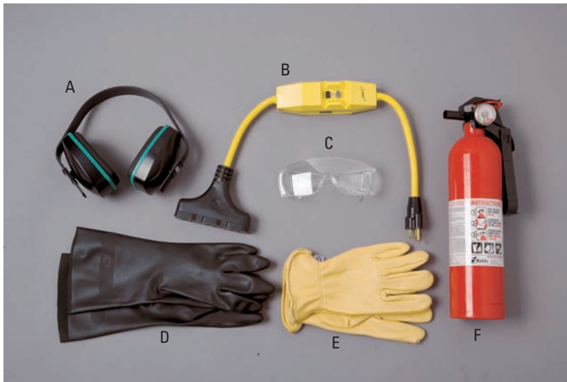
Figure 4-5: Necessary safety equipment.
