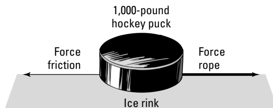
Figure 5-6: Pulling a 1,000-pound puck with a rope to exert equal force on both ends.
