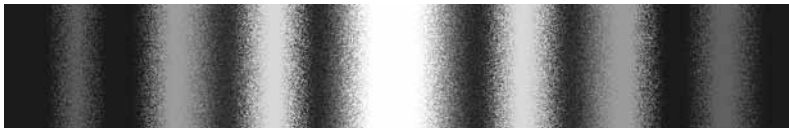
Figure 13-4: The interference pattern of electrons sent through dual slits.
