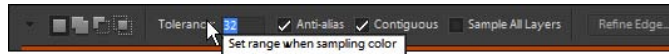
Figure 2-4: The Tolerance value can be changed to select a wider or narrower range of pixels.
