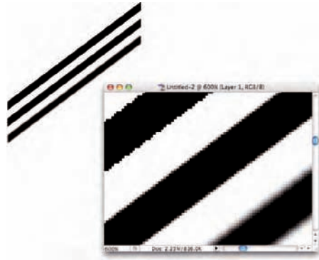
Figure 8-5: Anti-aliasing helps smooth the appearance of curves and diagonals.
