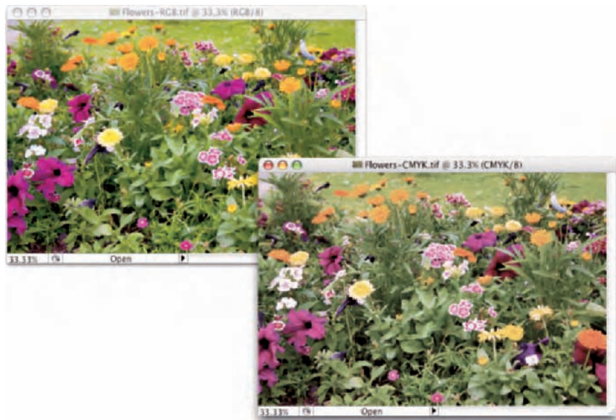
Figure 6-1: A wide-gamut image (on the left) and the same picture with a smaller gamut.
