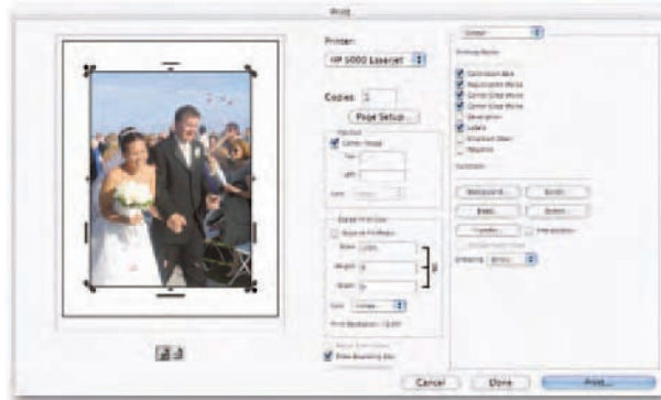
Figure 1-3: When printing color separations, be sure and check the necessary options in the Output section of the Print dialog box.
