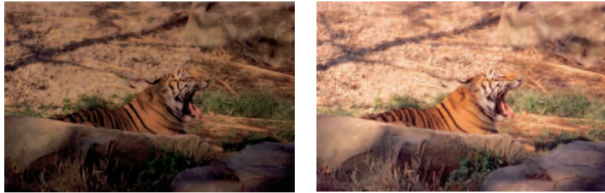
Figure 1-13: Applying the Levels command to a dark photo dramatically improves the contrast.
