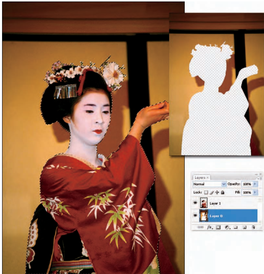
Figure 1-9: Cutting and pasting a selection from one layer to another leaves a transparent hole on the original layer.
