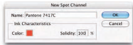
Figure 1-4: Adding an additional color separation in Photoshop requires creating a spot color channel first.
