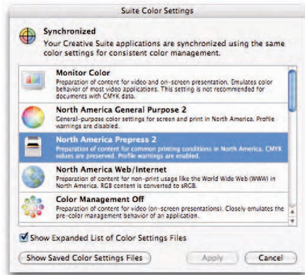
Figure 3-13: Getting consistent color among your Adobe Creative Suite applications is a matter of a few clicks in Adobe Bridge.
