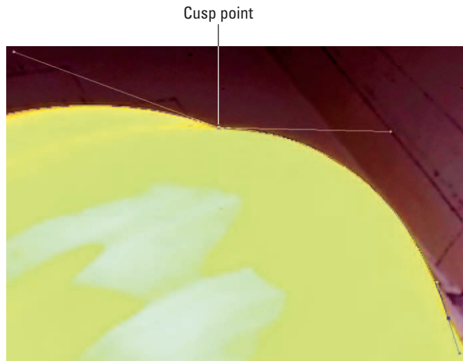
Figure 2-7: You can connect two curves that go in the same direction with a cusp point.
