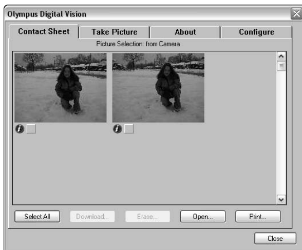
Figure 5-2: Transferring one or more photos to your PC with a TWAIN-compliant camera — in this case, an Olympus D-560.
