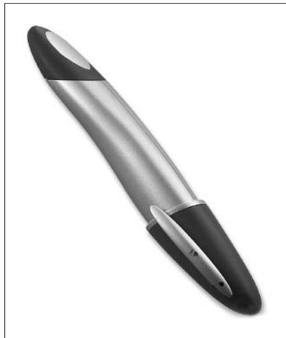
Figure 2-5: A digital pen is a specialized scanner.
