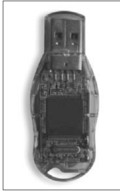
Figure 2-13: Carry 128MB in your pocket with a USB flash drive.
