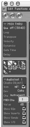
Figure 13-3: You assign a MIDI channel in Logic by clicking and holding the MIDI Channel selector in the Arrange window's track channel strip.
