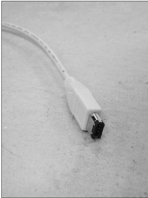
Figure 5-10: FireWire is a high-speed data transfer protocol.
