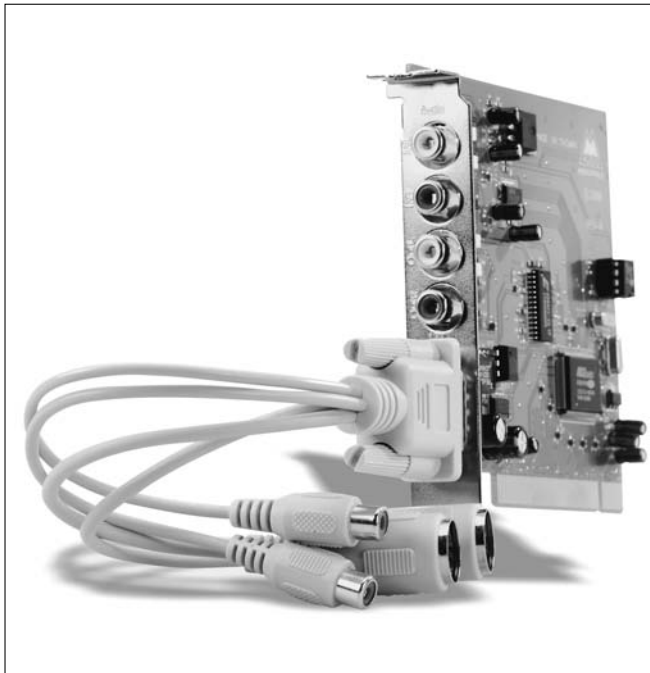
Figure 4-2: PCI interfaces like the M-Audio Audiophile 2496 often come with analog connectors.
