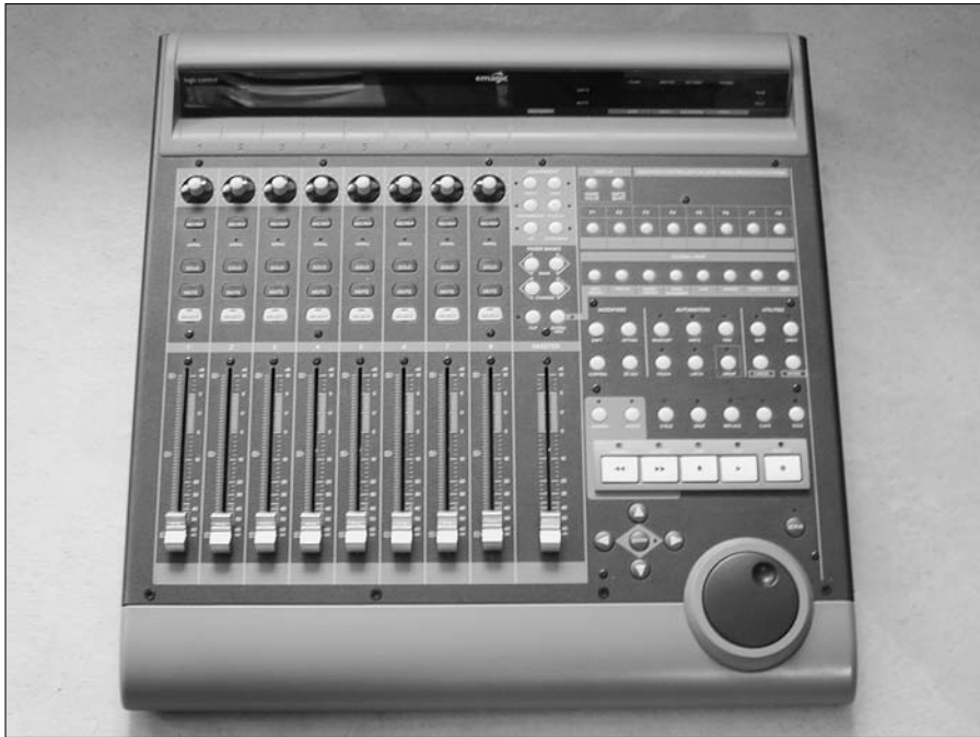
Figure 1-6: A computer-control surface offers you real knobs and faders and still uses the mixer that's part of your software.
