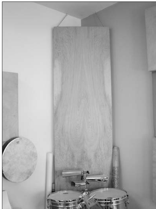
Figure 2-9: Put bass traps in the corners behind you to eliminate standing waves.
