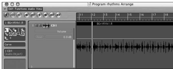
Figure 10-18: Regions are the visual representations of the audio you recorded for your song.
