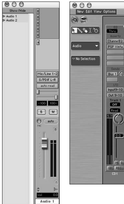
Figure 10-10: Your track's channel strip (in Pro Tools, left, or Logic, right) shows the level of your signal coming into your system.
