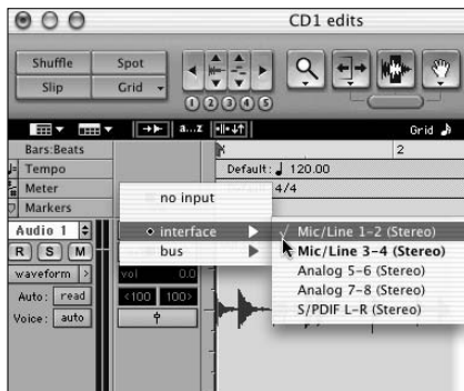
Figure 11-4: Assigning an input (or output) in Pro Tools is done by clicking and holding the Input or Output selector to open a contextual menu.
