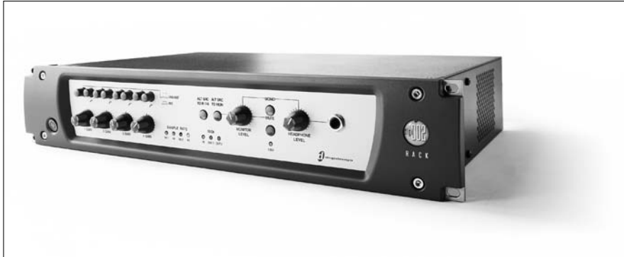
Figure 4-4: A FireWire interface, like the Digi 002, connects to the FireWire port in your computer.
