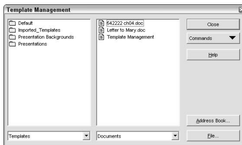
Figure 4-9: Use the Template Management dialog box to copy styles from one document or template to another.
