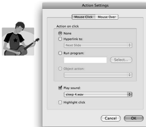
Figure 8-4: Using an action setting to play a sound when clip art is clicked.
