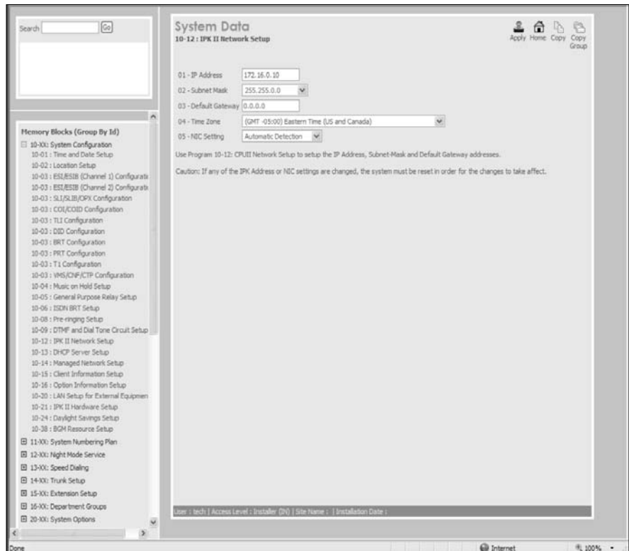
Figure 2-4: Changing the PBX system's IP address.
