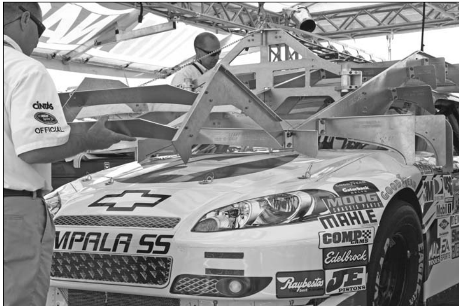
Figure 6-2: NASCAR inspectors fit tem- plates to a car during inspections.
