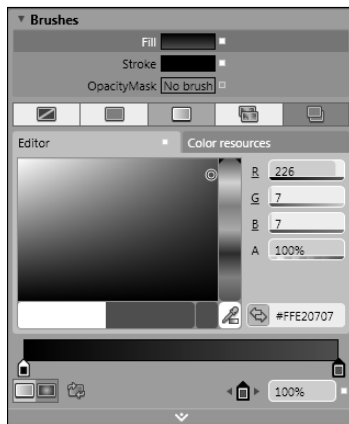
Figure 3-15: Setting gradient properties.
