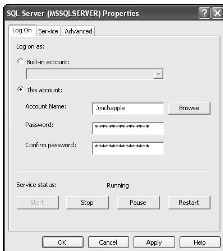
Figure 3-4: SQL Server Service properties.
