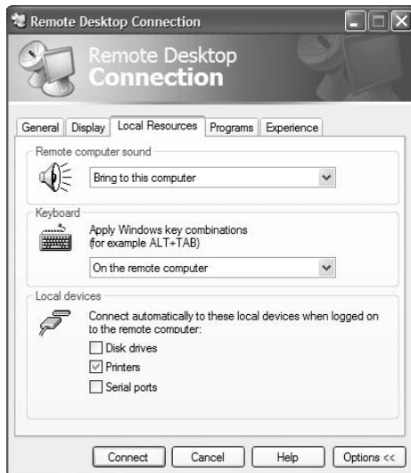
Figure 14-11: Perform automatic resource mapping to make local resources available for use.
