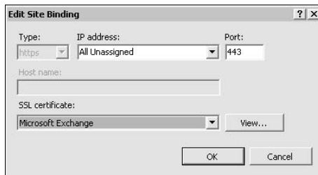
Figure 4-25: Add the correct SSL certificate to the binding.
