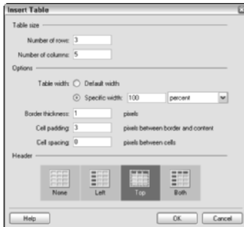
Figure 2-8: The Insert Table dialog box asks for enough information to create a basic HTML table.
