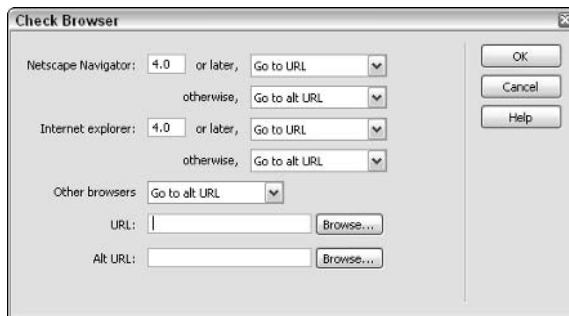
Figure 9-15: The Check Browser dialog box lets you direct users to different URLs based on which browsers they're using.
