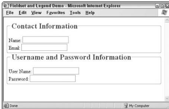
Figure 7-14: The <fieldset> and <legend> tags format form data in a unique way.
