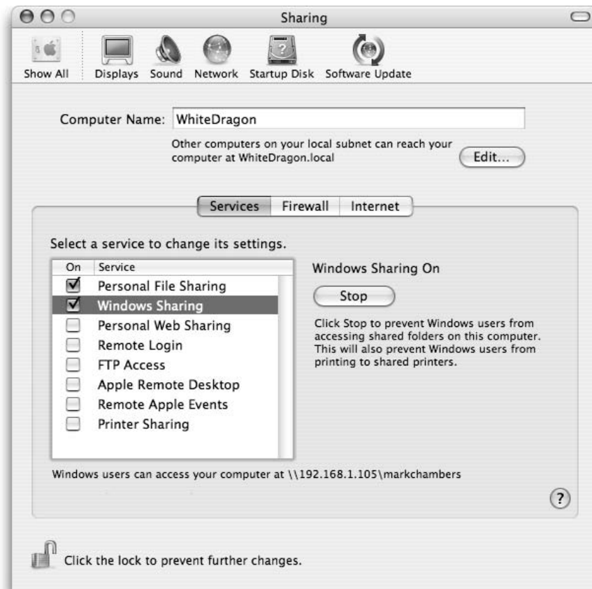
Figure 3-18: These settings control file sharing, FTP access, and printer sharing (among others).
