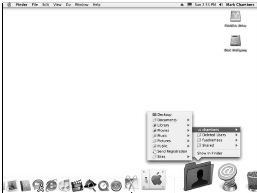
Figure 2-5: Click and hold on a folder in the Dock to display a Dock menu with its contents.
