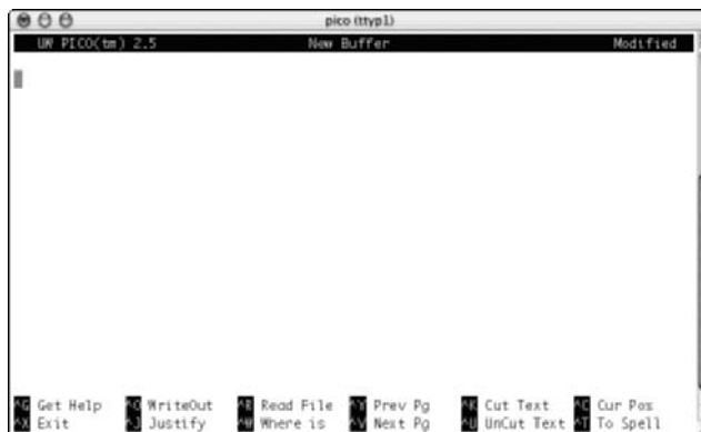
Figure 1-12: The pico program is a full-featured text editor built into the command line.
