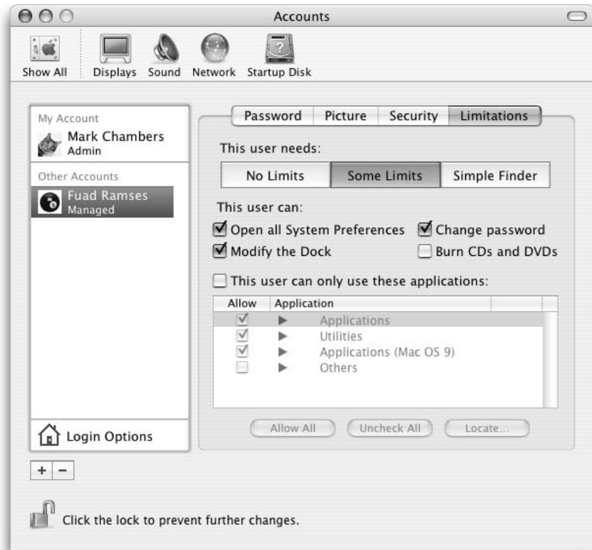
Figure 5-4: You can restrict access to all sorts of functions within a Standard account.
