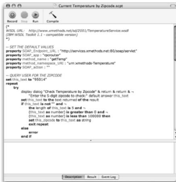
Figure 2-4: Click the Run button to execute a script that's loaded in the Script Editor.
