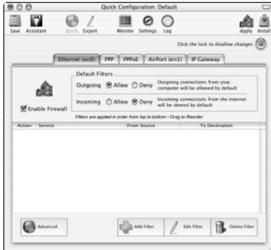
Figure 6-3: BrickHouse provides another route for configuring IPFW.
