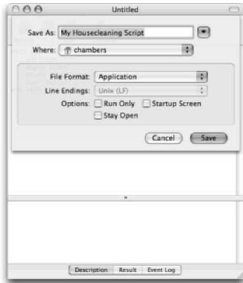
Figure 2-7: Save your script as an application so that you can run it again later.
