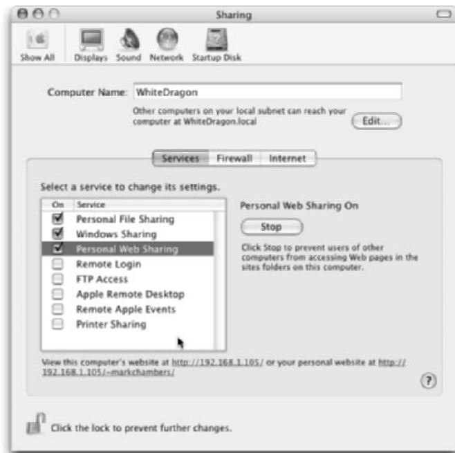
Figure 4-6: Start your Web server with only one click in the System Preferences.
