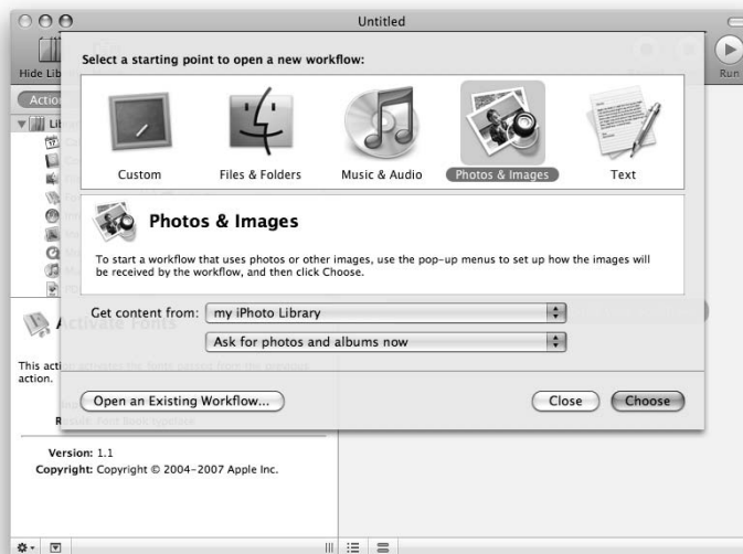
Figure 16-5: Choose a starting point and Automator will assist you; choose Custom to start a workflow from scratch.
