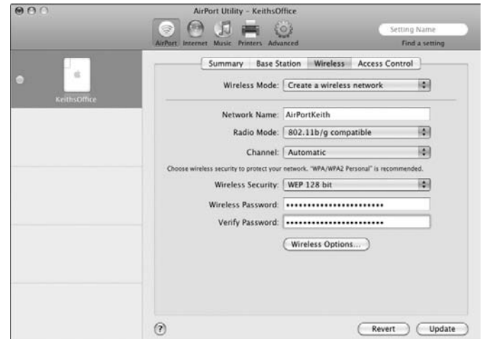
Figure 20-10: The 128 bit WEP password should be exactly 13 characters long.
