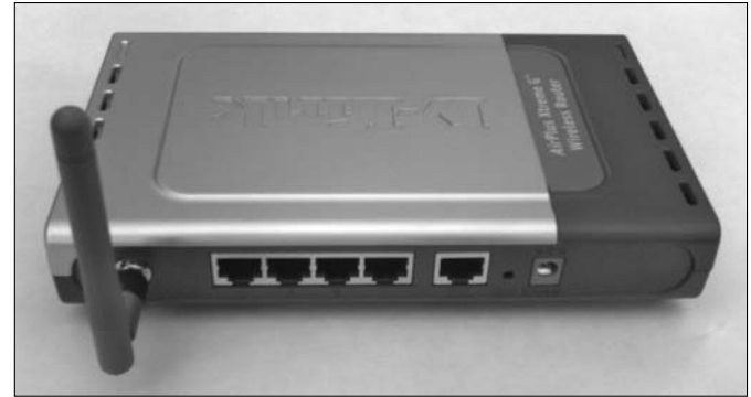
Figure 22-1: This router has multiple Ethernet ports.
