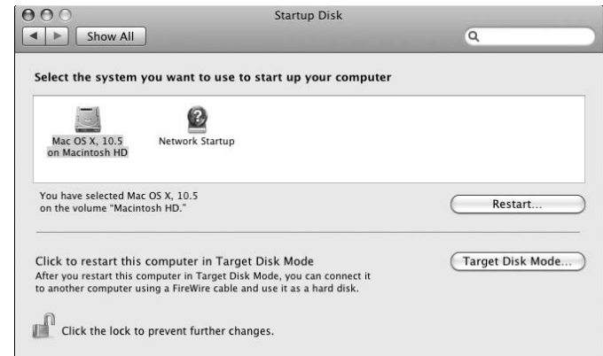
Figure 4-5: Select the disk or operating system that you want to use when the computer starts.
