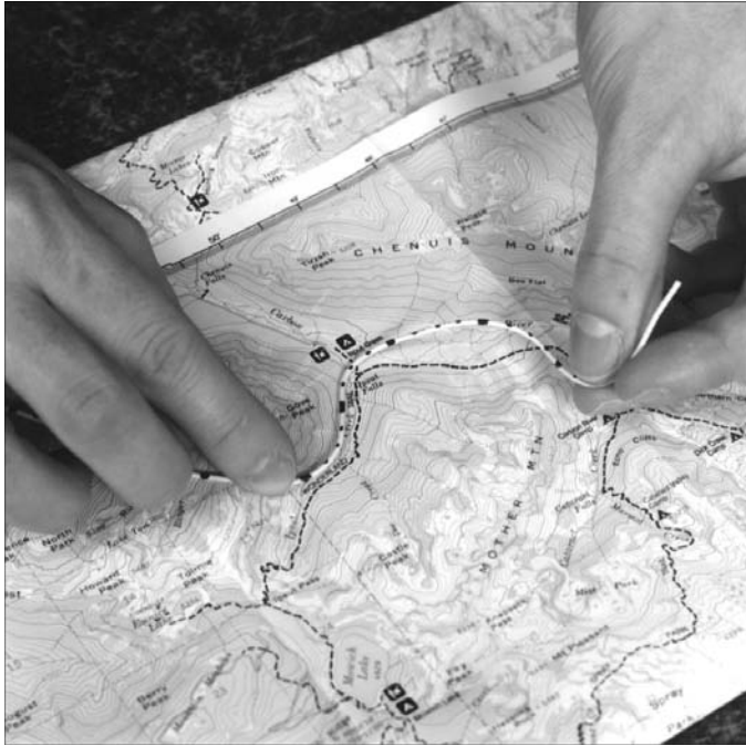
Figure 2-3: Measuring trail distance with a piece of electrical wire.
