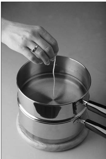
Figure 5-4: To prime your wick, just melt your wax, dip your wick, and let it cool.
