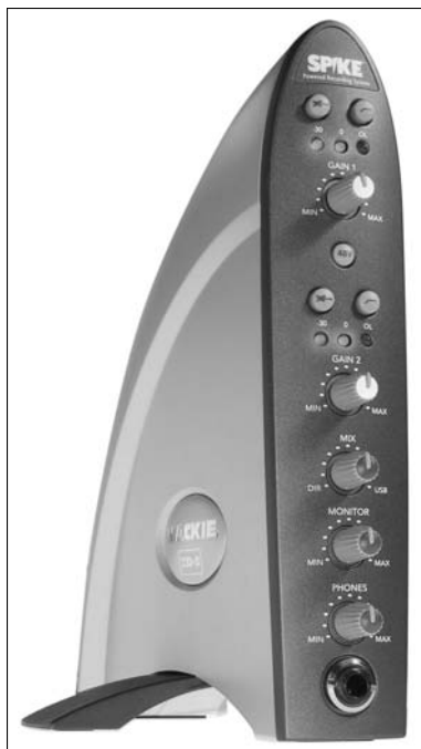
Figure 2-5: A USB interface connects to your computer's USB port.
