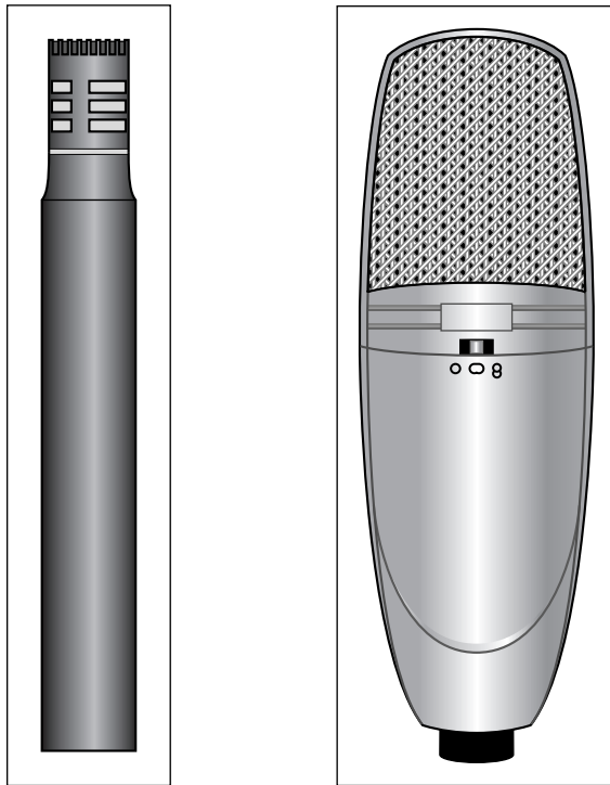
Figure 6-2: Condenser mics can have either small or large diaphragms.
