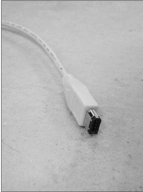
Figure 3-9: FireWire is a high-speed data- transfer protocol.
