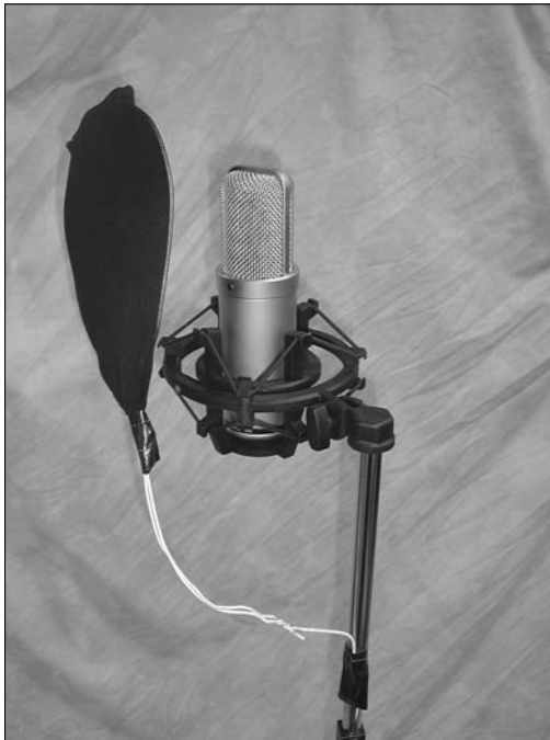
Figure 6-8: You can make a pop filter out of a coat hanger and a pair of tights or panty hose.
