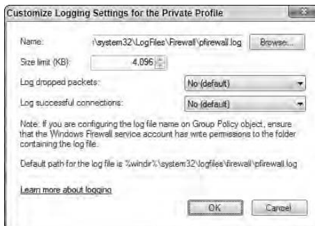
Figure 12-12: Set logging options for creating an audit trail of the firewall's activity.
