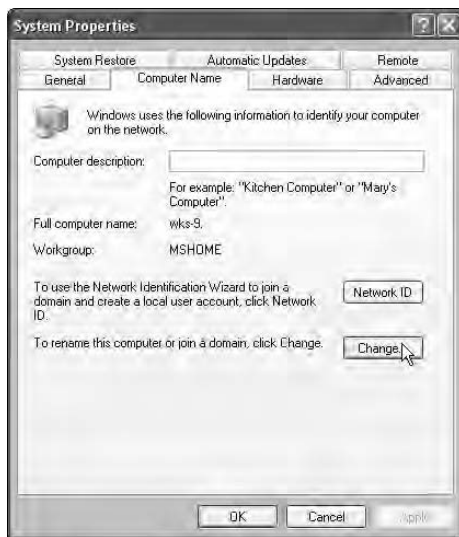
Figure 6-1: Your computer name and its workgroup are stored on the Computer Name tab of the System Properties dialog box.
