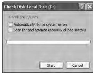
Figure 14-5: Configure the way you want the error checking tool to perform its task.
