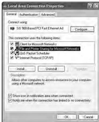
Figure 9-1: In Windows XP, enable File and Printer Sharing in the Properties dialog box of your Local Area Connection.
