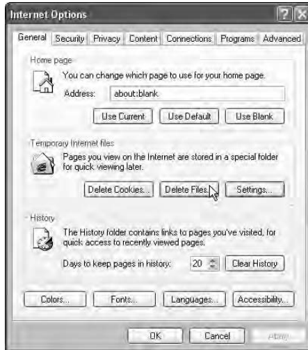
Figure 14-1: Remove unneeded files and configure options in the IE6 Internet Options dialog box.
