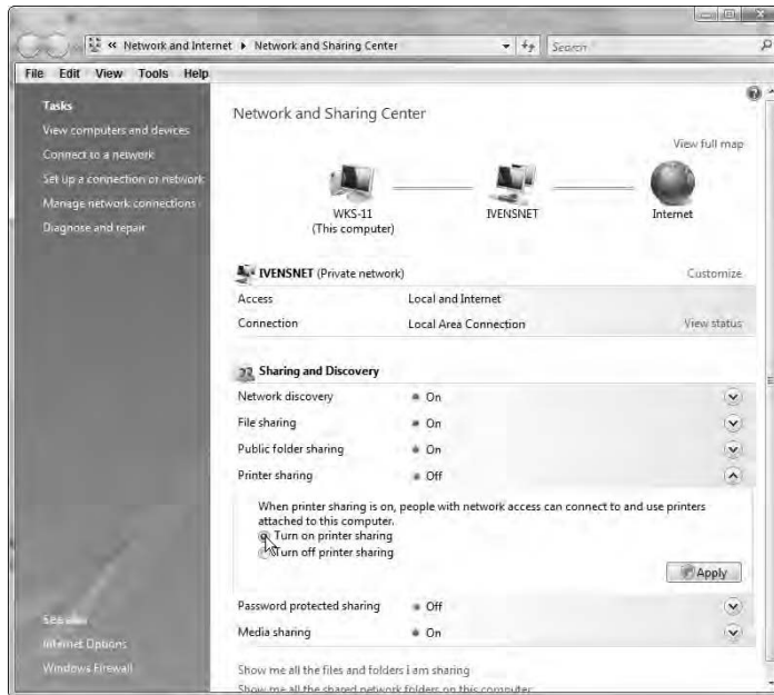
Figure 9-2: Enable the printer sharing feature in the Network and Sharing Center window.
