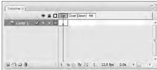
Figure 8-2: The Flash symbol-editing mode for buttons displays a Timeline with four frames.
