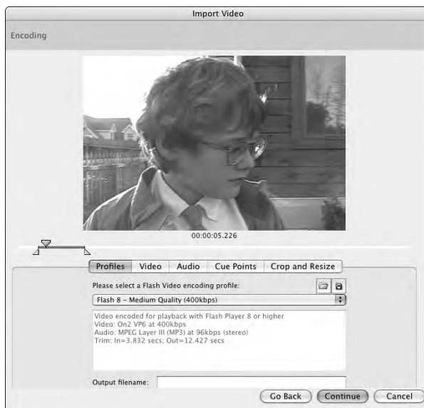
Figure 11-5: In the Encoding pane of the Import Video dialog box, you can select how much compression to apply to your video clip.
