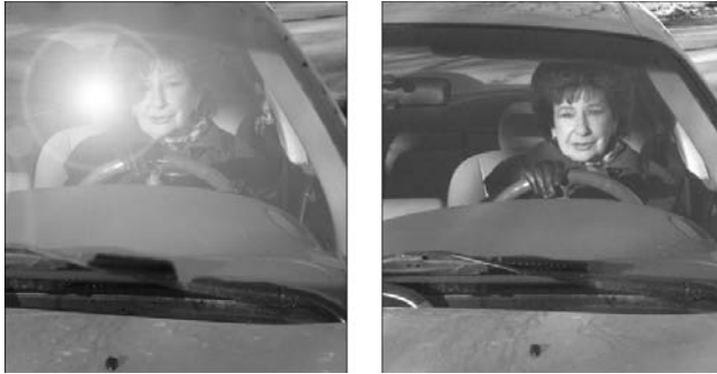
Figure 10-6: Without polarizer (left) and with polar- izer (right).
