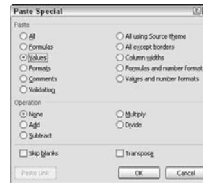
Figure 3-10: Paste only the value, not the formula with the Paste Special feature.
