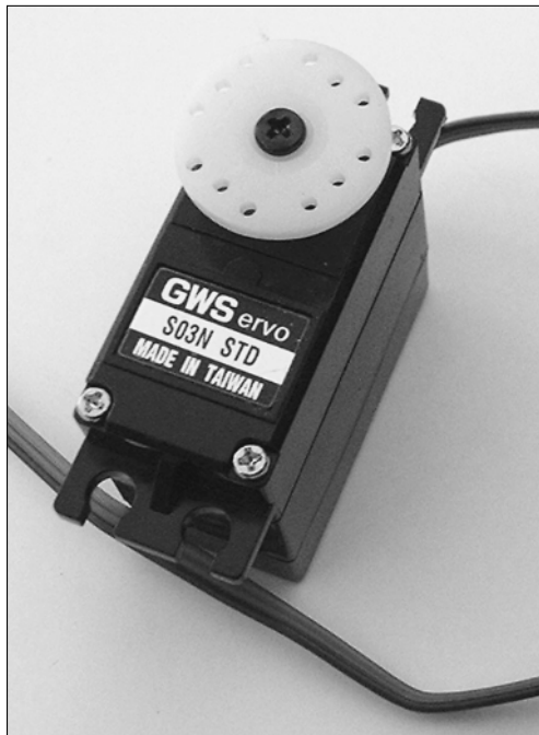
Figure 15-11: A typical standard- size R/C servo motor.
