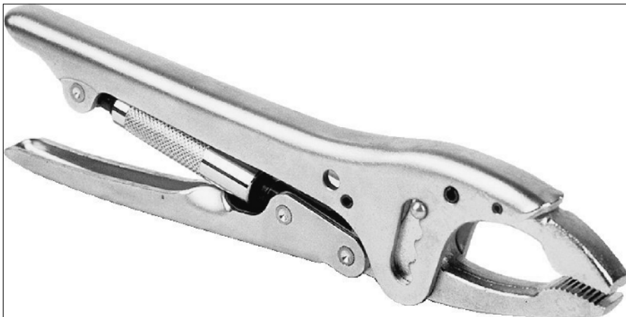
Figure 3-5: Locking pliers work like regular pliers, but they have a locking mechanism to keep them closed in position.
