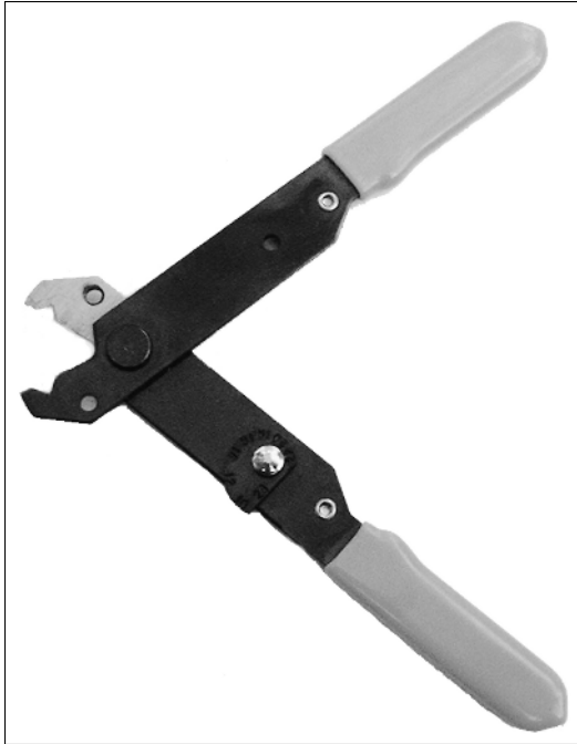
Figure 3-2: A combination wire cutter and stripper.
