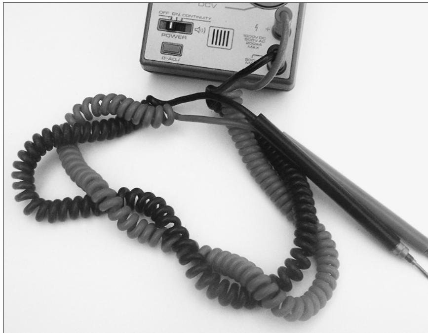
Figure 9-5: Coiled leads stretch out during use but shrink back to normal size for storage.
