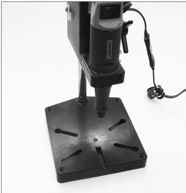
Figure 12-7: Use a small drill press to drill the holes in your PCB.
