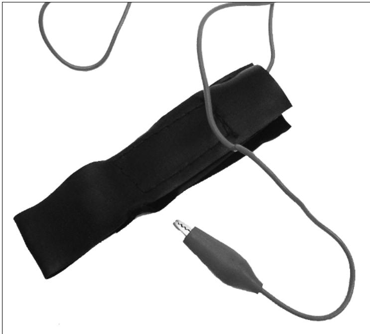
Figure 2-1: An anti-static wrist-strap reduces or eliminates the dangers of electrostatic discharge.
