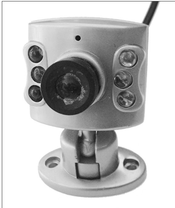
Figure 14-6: This miniature camera can see in the dark, thanks to its six infrared-emitting diodes.
