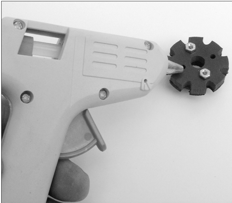
Figure 3-8: A hot-melt glue gun quickly fastens things.
