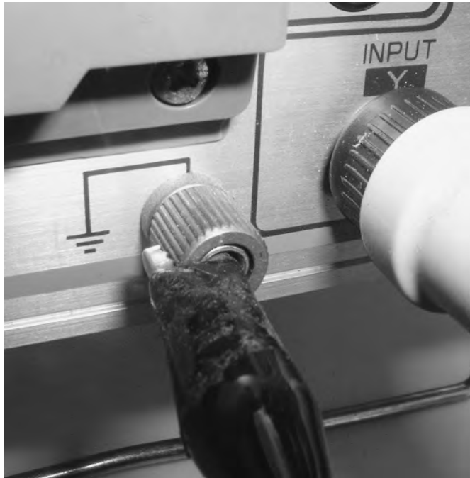
Figure 10-10: Connect the ground of the probe to the ground connection on the scope.
