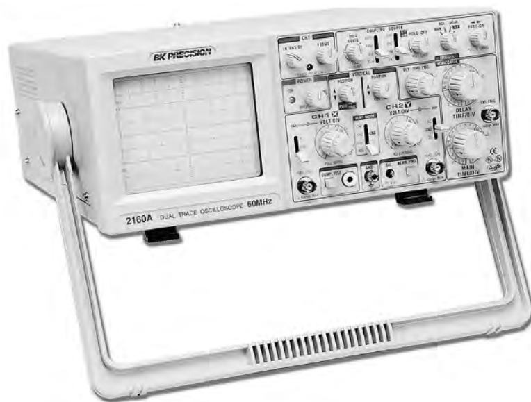
Figure 10-7: A bench scope sits on your worktable and is completely self-contained.
