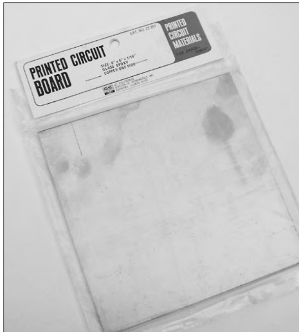
Figure 12-1: A printed circuit board is made of copper and an insulating backing.
