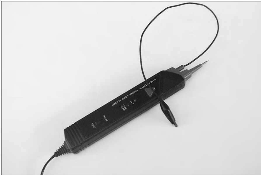
Figure 16-1: Logic pulsers feed a short signal burst into a circuit.
