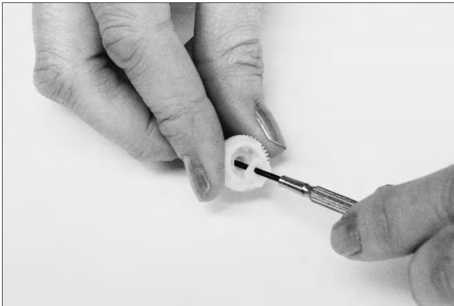
Figure 15-18: Use a small screw- driver to remove the potentio- meter shaft clip.
