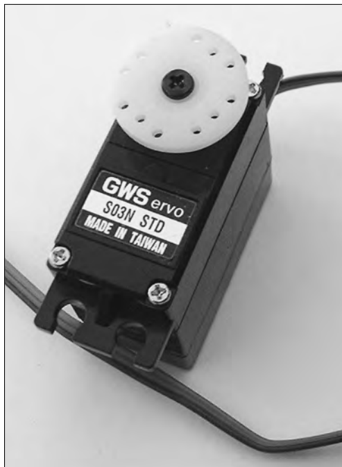
Figure 15-11: A typical standard- size R/C servo motor.
