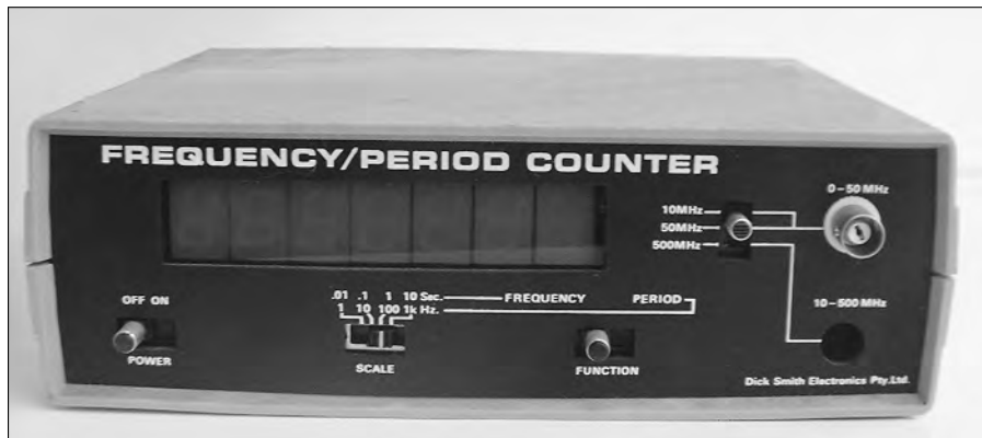
Figure 16-2: A digital frequency counter adds up frequencies.
