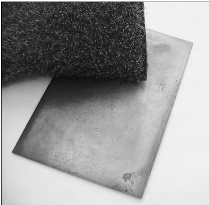
Figure 12-3: The copper clad must be spotless before you make a circuit on it.
