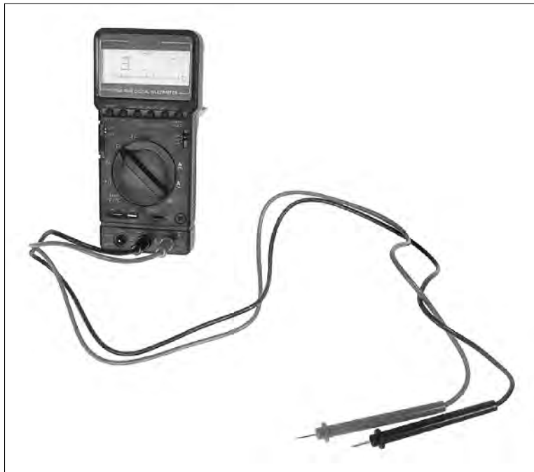
Figure 9-7: On automatic ranging multimeters, setting the desired test function automatically selects the range.
