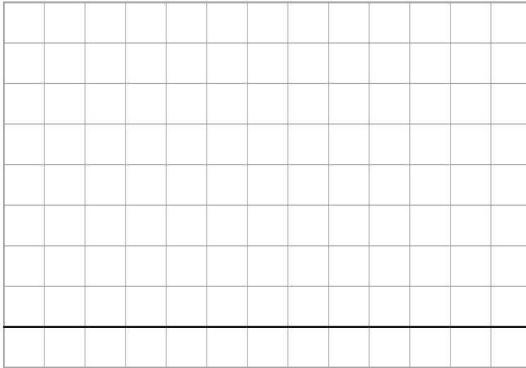
Figure 10-11: Adjust the Vertical Position knob so that the beam sits on the bottom of the grid.
