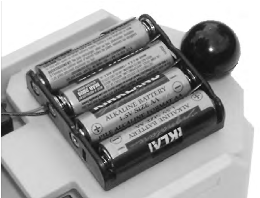
Figure 5-5: Four 1.5-volt batteries tucked into a battery holder produce about 6 volts.
