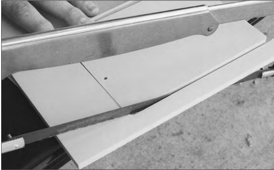
Figure 15-2: You can cut the Rover pieces using a hacksaw.
