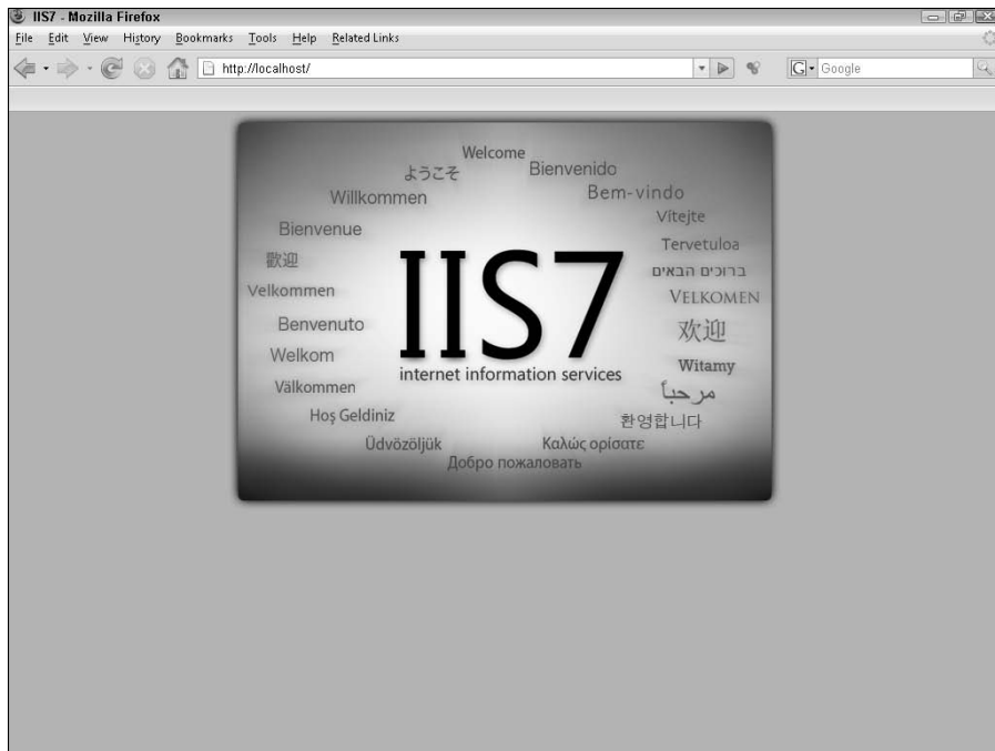
Figure 14-3: You can test your local server by entering http://localhost into a Web browser.
