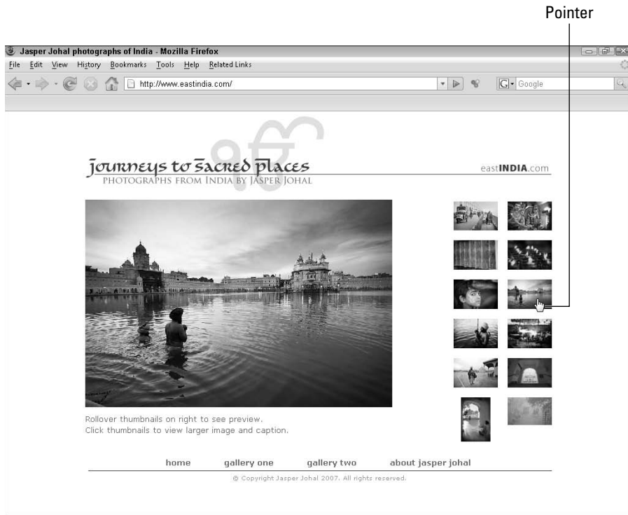
Figure 10-4: When you preview a behavior in a browser, you can see the effect of the Swap Image behavior when the cursor is rolled over an image.
