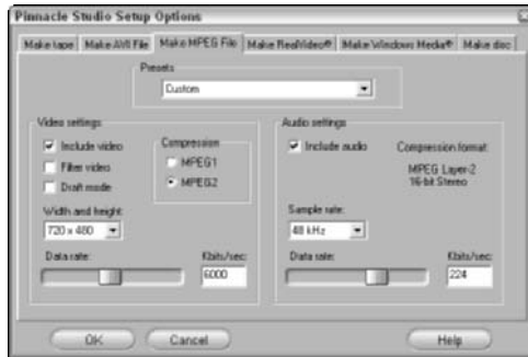
Figure 13-4: The Setup Options dialog box in Pinnacle, with its MPEG tab visible.
