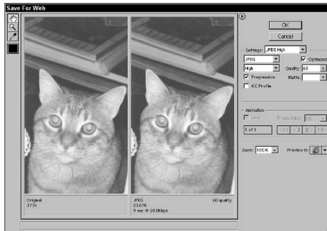
Figure 21-3: You can save an image especially for Web display in Photoshop Elements.
