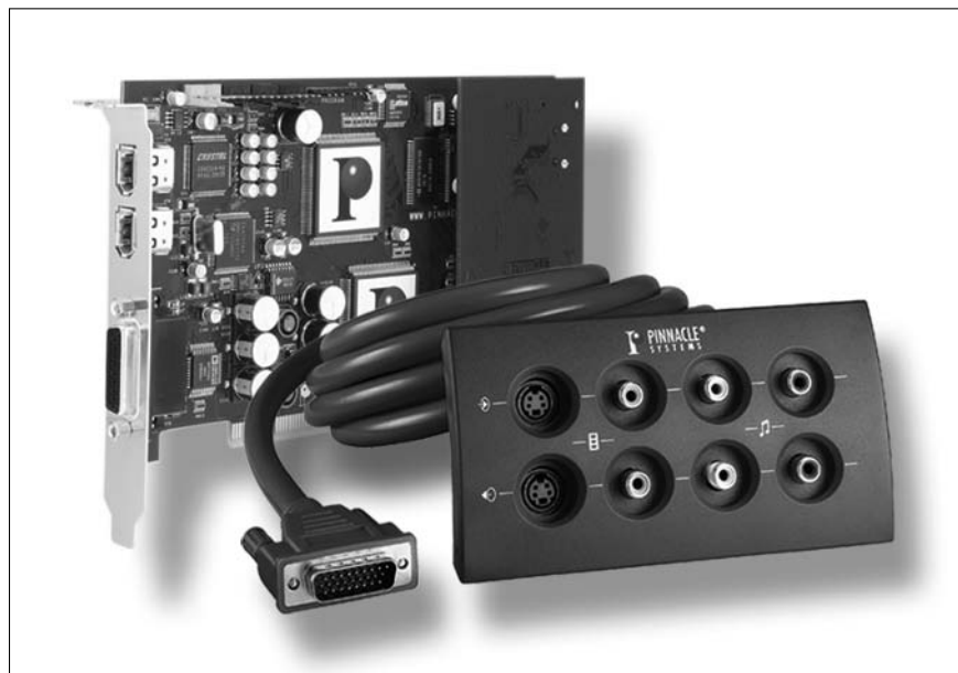
Figure 3-7: Some capture cards put all their audio and video connectors on a breakout box.
