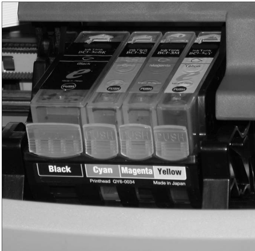
Figure 5-1: Replacing one-color ink tanks is far cheaper than replacing a whole color cartridge.
