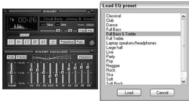
Figure 3-5: Click the EQ button and then the Presets button to see Winamp's equalizer settings for different environments and moods.
