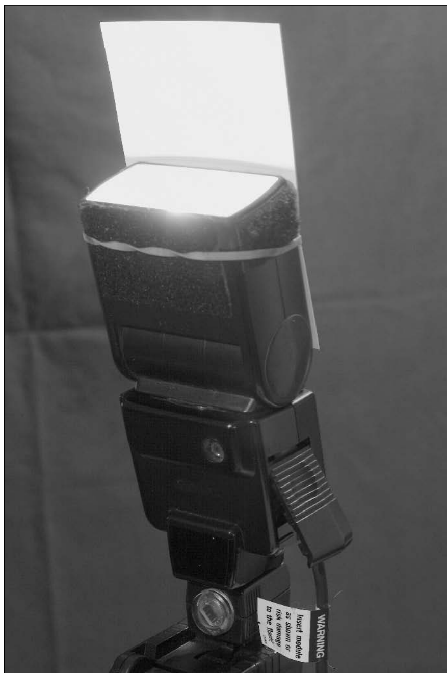
Figure 9-6: Need fill lighting? Just use an index card and a rubber band.
