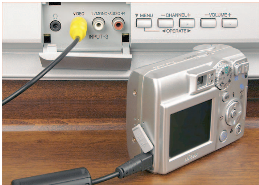
Figure 10-11: Many cameras enable you to send video signals from the camera to your TV, VCR, or DVD player for playback.
