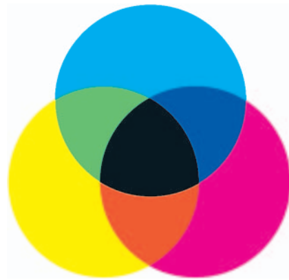
Figure 2-15: The print color model is based on cyan, magenta, and yellow ink.
