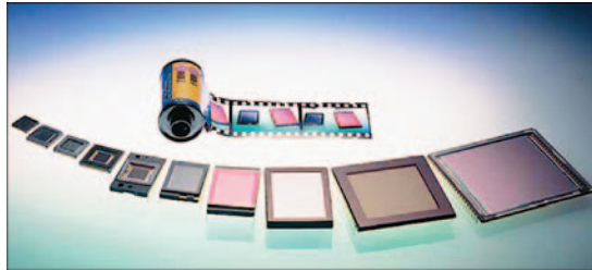
Figure 2-1: Imaging sensors do the work of film in digital cameras.
