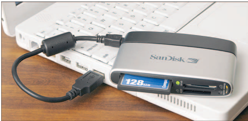
Figure 8-2: Just push the memory card into the matching slot on the card reader.
