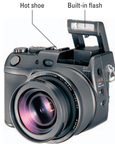
Figure 3-12: A hot shoe enables you to attach an external flash unit.
