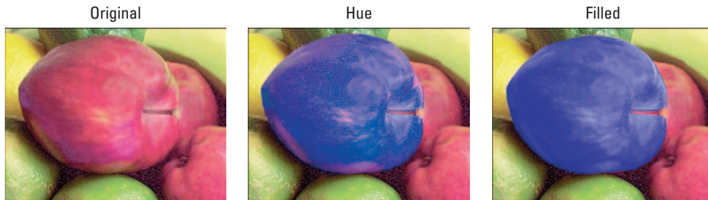
Figure 13-20: Changing colors via the Hue filter produces slightly different results than painting the pixels using the Color blending mode.
