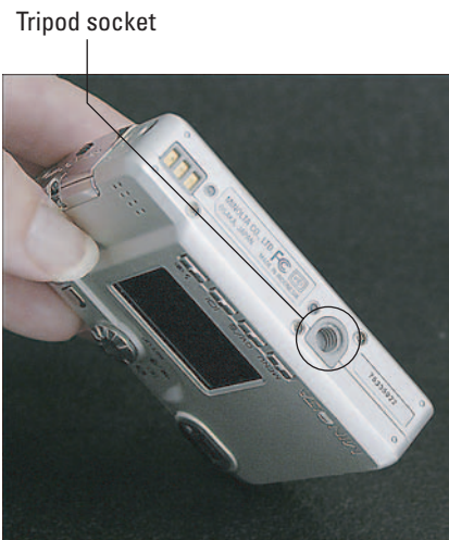
Figure 3-16: The screw socket on the bottom of the camera is for attaching a tripod.
