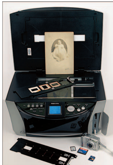
Figure 9-8: This all-in-one from Canon can print from a memory card or camera and also can scan prints, slides, and negatives.
