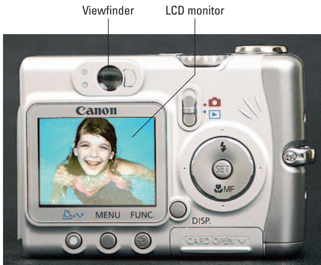
Figure 3-7: The LCD monitor enables you to review images immediately after you press the shutter button.
