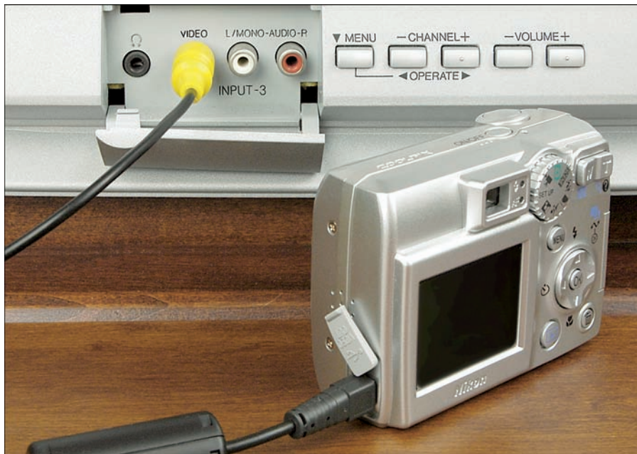
Figure 11-9: You can connect some cameras to a TV for picture playback.
