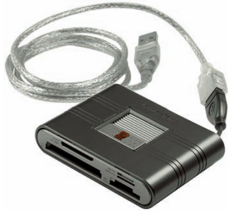
Figure 8-5: Just push the memory card into the matching slot on the card reader.
