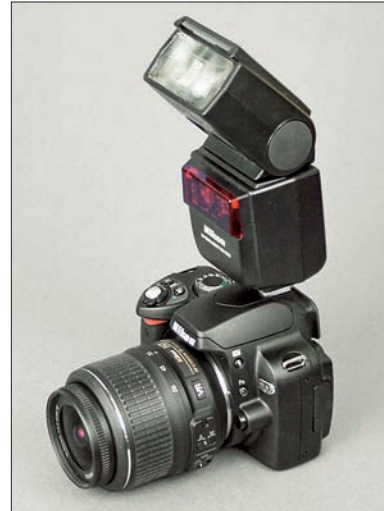
Figure 5-19: An external flash with a rotating head offers more flexibility and better illumination than a built-in flash.
