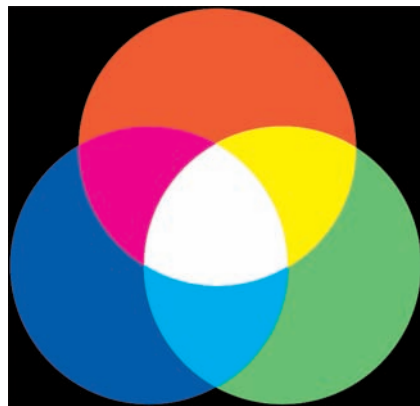
Figure 4-5: The RGB color model is based on red, green, and blue light.
