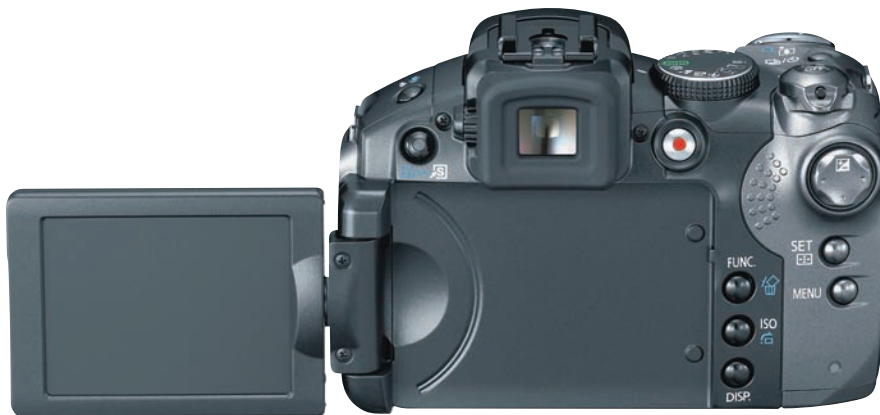
Figure 1-9: Some monitors can be adjusted to different viewing angles.
