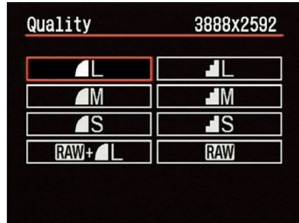
Figure 3-10: On some cameras, you set resolution and format together.
