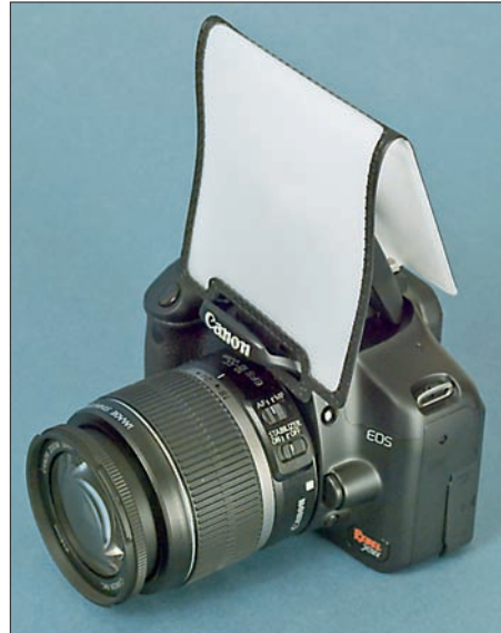
Figure 5-16: You can buy diffusers that soften the harsh light of a built-in flash.
