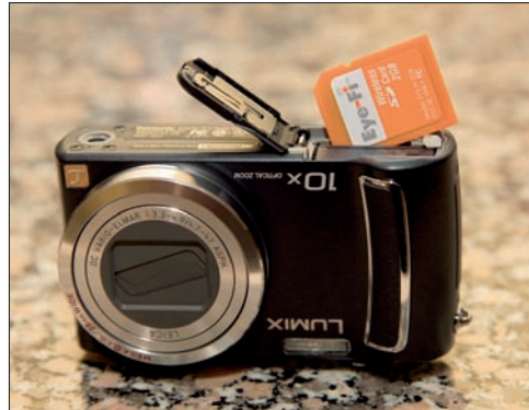
Figure 1-11: The Eye-Fi SD card combines a 2GB memory card with a wireless file transmitter.
