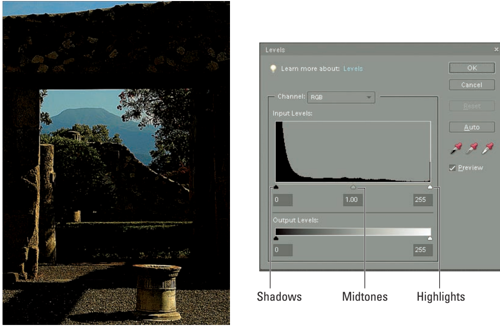
Figure 9-10: Drag the sliders under the histogram to adjust shadows, midtones, and highlights independently.
