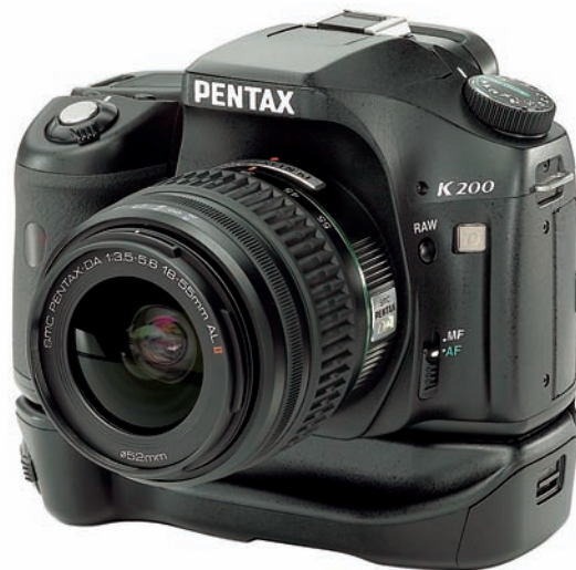
Figure 1-2: A dSLR camera can accept a variety of lenses and offers other higher-end capabilities.
