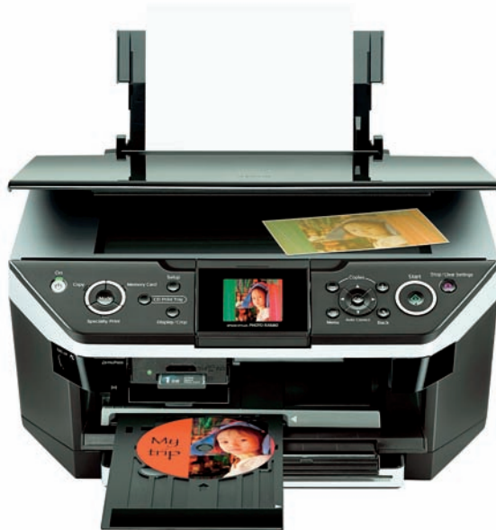
Figure 10-2: The Epson Stylus Photo RX680 is a scanner, copier, and photo printer that also prints onto CDs and DVDs.
