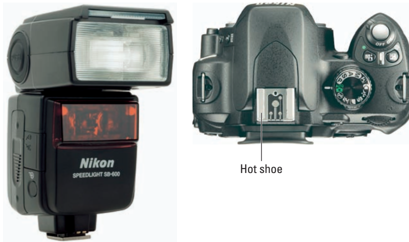
Figure 1-6: A hot shoe enables you to attach an external flash.
