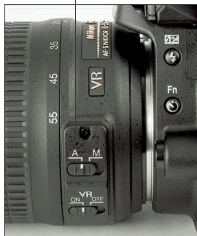
Figure 6-2: Some SLR lenses have a switch that sets the camera to autofocus mode.
