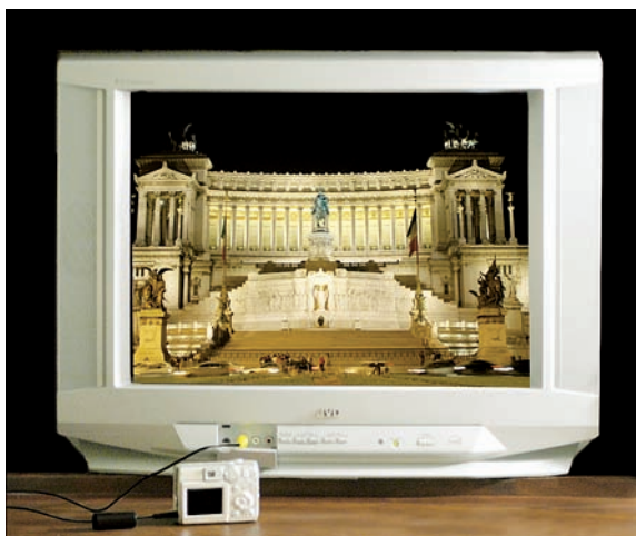
Figure 1-10: To view pictures on a TV, you need a camera that has a video-out port.
