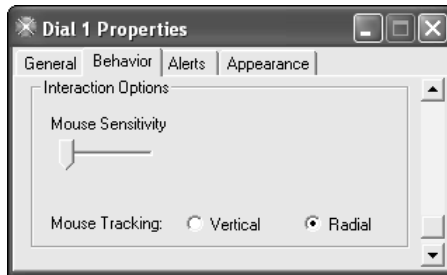
Figure 14-1: Set the Mouse Tracking property to Radial to allow circular mouse movement.
