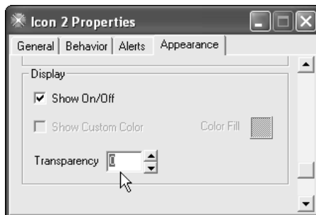
Figure 13-29: Setting the Transparency property to 0 makes an icon selector invisible.
