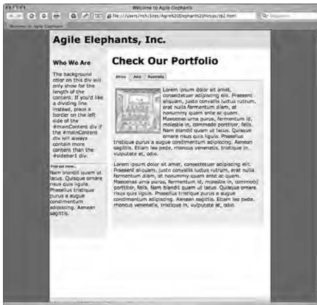
Figure 4-19: The collapsible panel was expanded when the user clicked the header.
