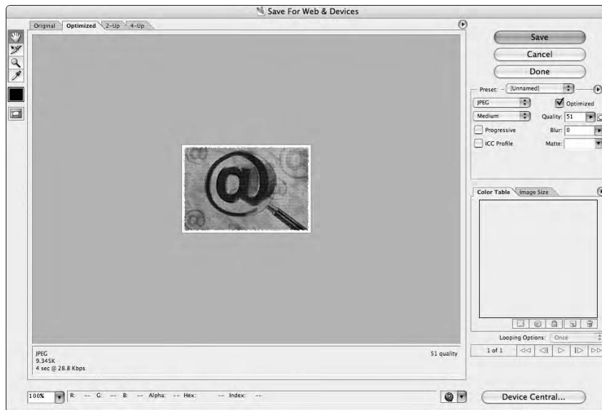
Figure 2-1: JPEG format allows you to determine the level of compression you want.
